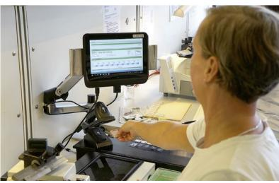
The system in action; the technician is scanning the barcode, which is on the side of the tissue block
