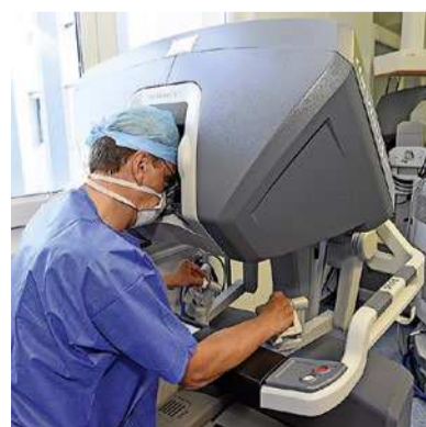
A surgeon controls the robot via a control console
